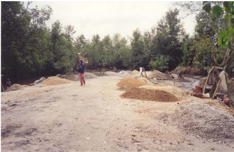
Picture 17: Second sand mine of fine to large grained sand mined from the mangroves at Youpwe
